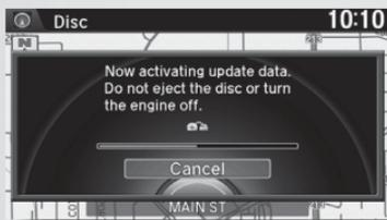
18. After the map update process is completed, a notification window appears to indicate the map update is complete. The system will then automatically reboot to activate the map data. **Do not eject the DVD or turn off the engine.**
