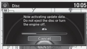
**Note:** If you eject the Disc or turn off the engine at this point, the system will discard the current update progress and start again from the beginning once the engine is restarted.
