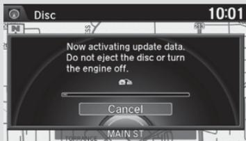
**Note:** Do not eject the Disc or turn off the engine during the map update process. If "Cancel" is pressed during the map update process you will receive error message **E3**, located in the error message section of this instruction booklet. Select "Yes" and message **E5** appears to confirm the cancellation of the update process.
